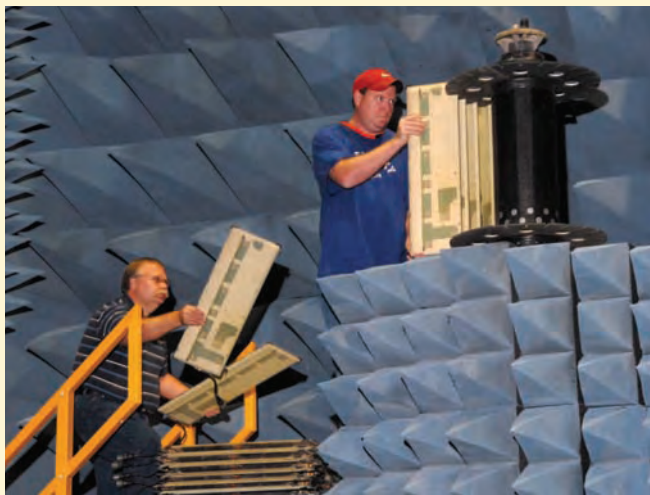
Figure 1 | LCMR technicians set up an AN/TPQ-48 for testing in the simulator's anechoic chamber. U.S. Army photo by Steve Grzedzinski.
