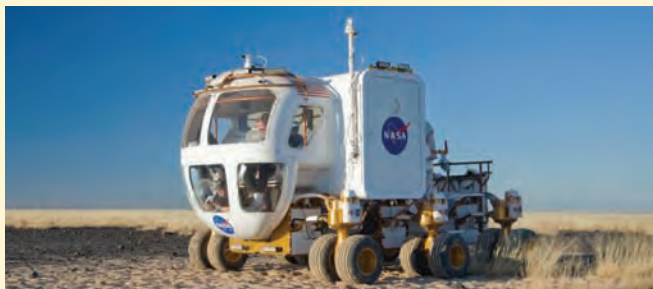
Figure 3 | Lunar Electric Rover (LER), created by Johnson Space Center, is destined to transport astronauts on Mars or the moon. Photo by NASA/Regan Geeseman
