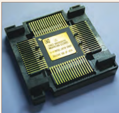
Figure 1 | An Intel 186 high-performance, low-power processor ideal for embedded applications is available through the Rochester Electronics Extension-of-Life process.
